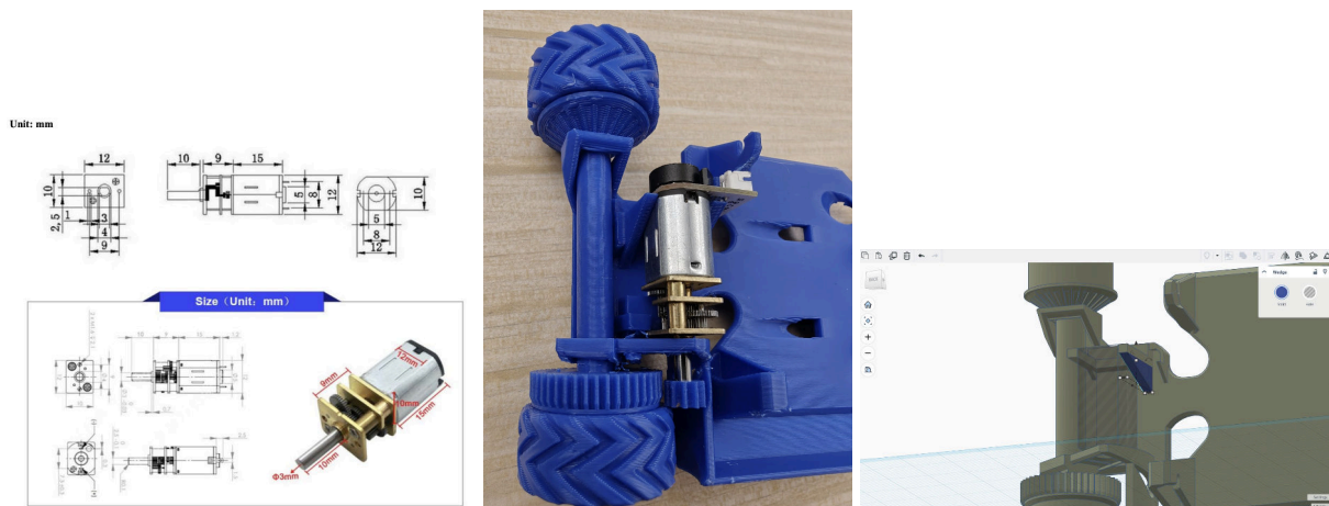
Figure 11: Motor integration: datasheet, 3D model, and actual motor placement
