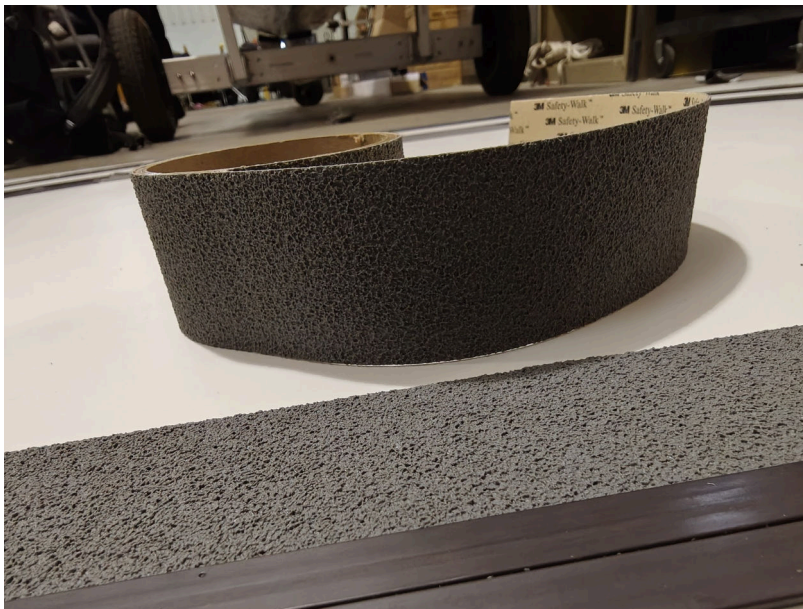
Figure 20: Grip tape applied along the track perimeter to increase friction
