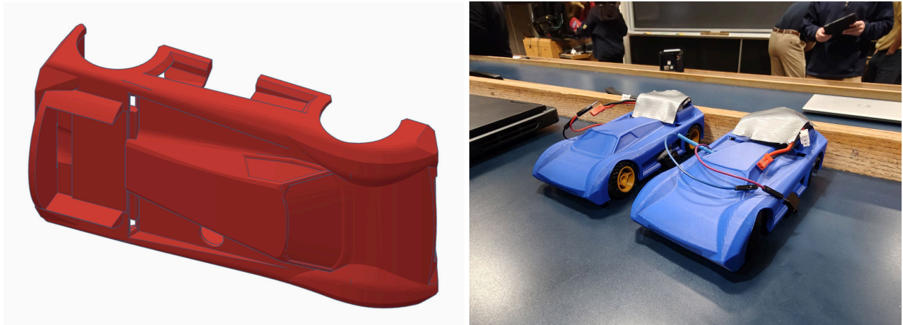
Figure 14: Updated car shell showing battery compartment, switch gap, and expanded wheel well
