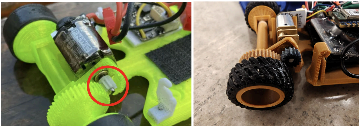
Figure 13: Pinion gear: Old (left) vs. New (right)
